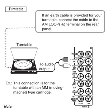
Any turntables incorporating a small-output cartridge such as an MC (moving-coil) type must be connected to this receiver through a commercial head amplifier or step-up transformer. Direct connection may result in insufficient volume.
